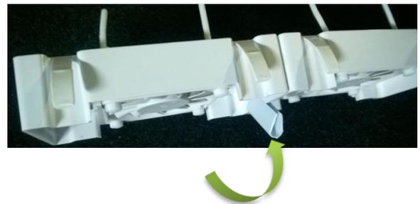
6. Slide the connected modules from the radiator's bottom up between its panels. During mounting, please pay particular attention to direct the fan modules with the label facing upwards. This will ensure the proper air flow direction.
